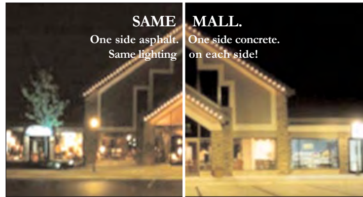
Concrete parking delivers enhanced safety: With three times the reflectivity of asphalt, concrete parking requires less lighting, reducing costs by up to 30%, while providing enhanced safety.
